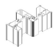
Normal and High Rise Interlock configuration for **600Pa (A0)** for sizes 1,5m to 6,0m and **1000Pa (A1)** for sizes up to 2,1m OX and 4,2m OXXO.
