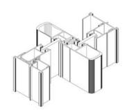
High Rise and High Rise Interlock configuration for **1500Pa** (**A2**) for sizes 2,1m to 6,0m and **2000Pa** (**A3**) for sizes up to 2,1m OX and 4,2m OXXO.
