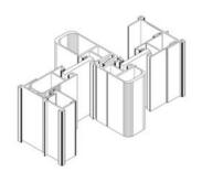
Intermediate and High Rise Interlock configuration for **1000Pa (A1)** for sizes 2,4m to 6,0m and **1500Pa (A2)** for sizes up to 1,8m OX and 3,6m OXXO.
